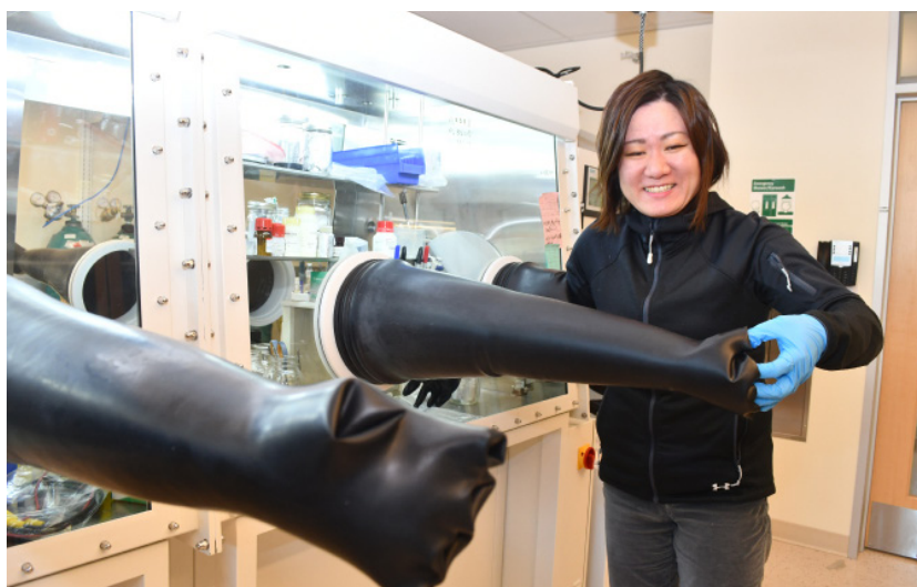
Assistant Professor of Chemistry Niya Sa puts her hand in the oxygen-free Glove Box she uses for her battery research.
